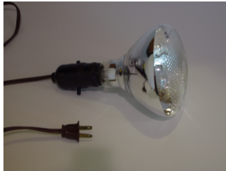
Non-conforming – exposed bulb
